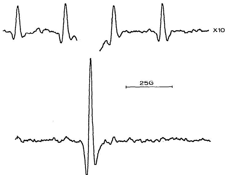
Fig. 2. The second-derivative ESR spectrum of \text{Cr}(\text{CO})_2\text{-}(\text{PQ})_2 in toluene at 25^\circ\text{C} . The upper insert shows the hyperfine lines of Cr isotope ( ^{53}\text{Cr} : 9.54%, I = 3/2 ).
